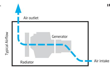
Cooling air passes nearly straight through - conventional sound reduction
