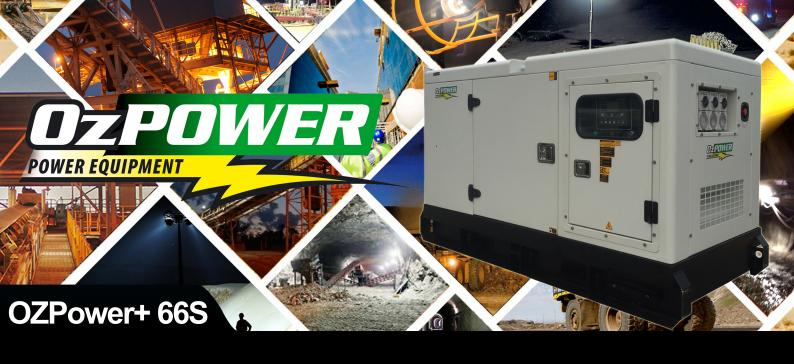
Model OZGPC60S Speed 1500 RPM Phase/Voltage 3, / 415 Frequency 50 Hz Power Factor .8 Stdby Power 66kVA / 52.8kW Prime Output 60kVA / 48kW Noise Level (dBA @ 7 m) 70.5dB(A) Fuel Run Time 24 Hours Length 2.67 m Width 1.08 m Height 1.865 m Weight 1490 kg
